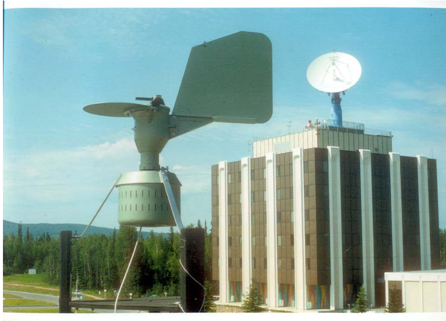
Figure 1. The Burkard 7-day volumetric sampler. (Photo courtesy of J Anderson).
